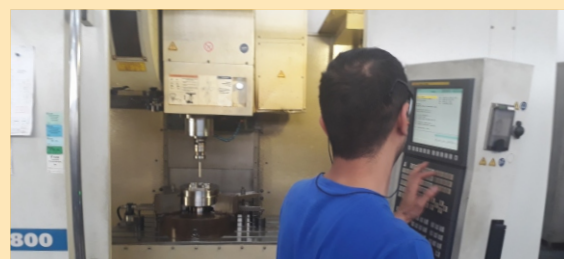
Figure 5. CNC machining of the SMT-20 connection block
