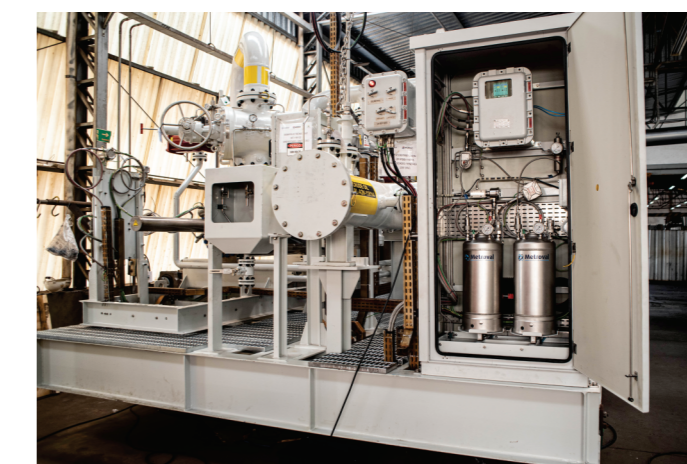
Sample receivers with scales assembled in Stainless Steel cabinet or GRP (Glass Fiber Reinforced Polyester) with a heating system to preserve the samples temperature in order to maintain the liquid phase.
