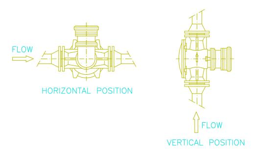
WARNING: Never install the Oval Gear Meter as shown in the figure below.
